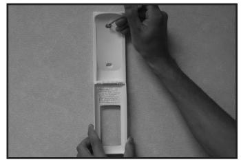
Figure 12.6 Mounting Remote Control Housing
